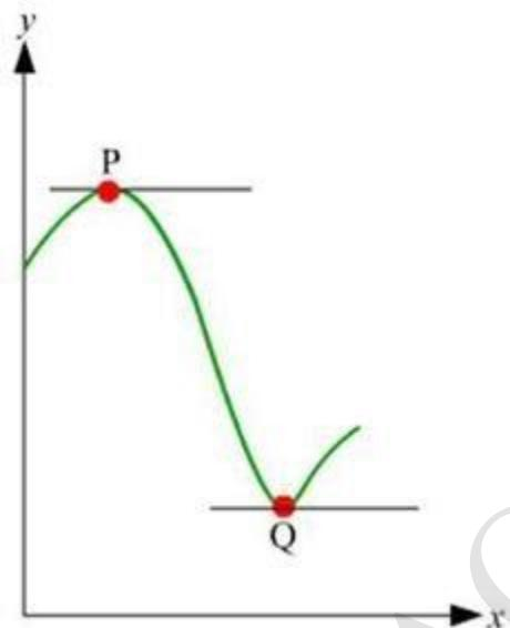
At the points P and Q the tangents to the curve is parallel to the x-axis.
