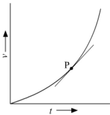
$a = \lim_{\Delta t \rightarrow 0} \frac{\Delta v}{\Delta t} = \frac{dv}{dt}$  = slope of the tangent at point P
